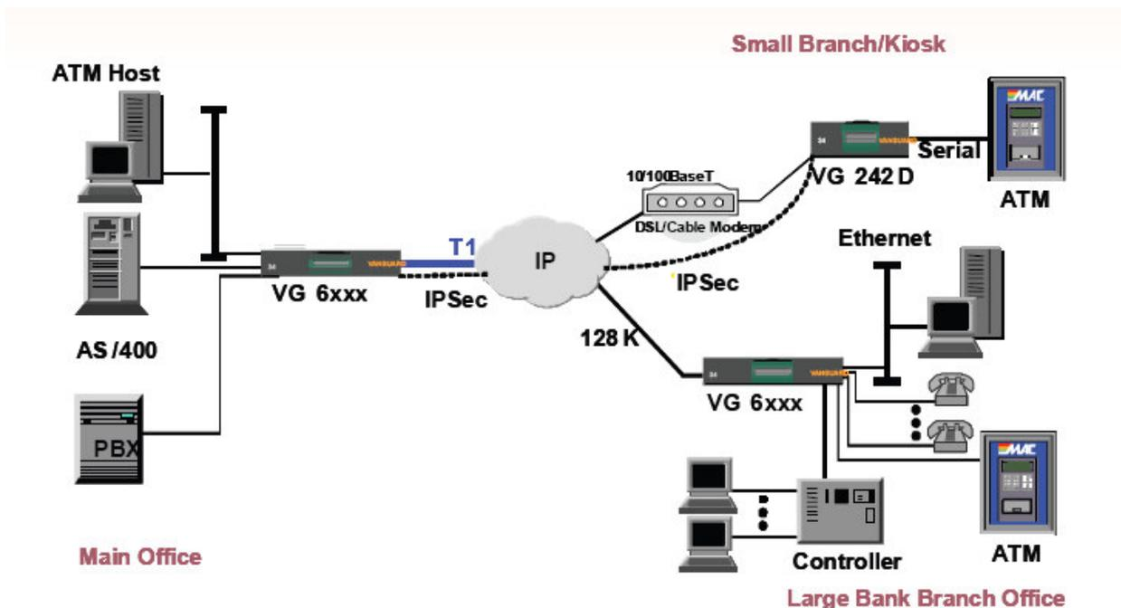
This diagram illustrates how the VG 242D fits into a bank application deploying another Vanguard portfolio product: the multi-service 6400 series router. The Vanguard 242D, in combination with the VG34x, 6400 and 7300 series products, enables a complete product solution for enterprise customers.
