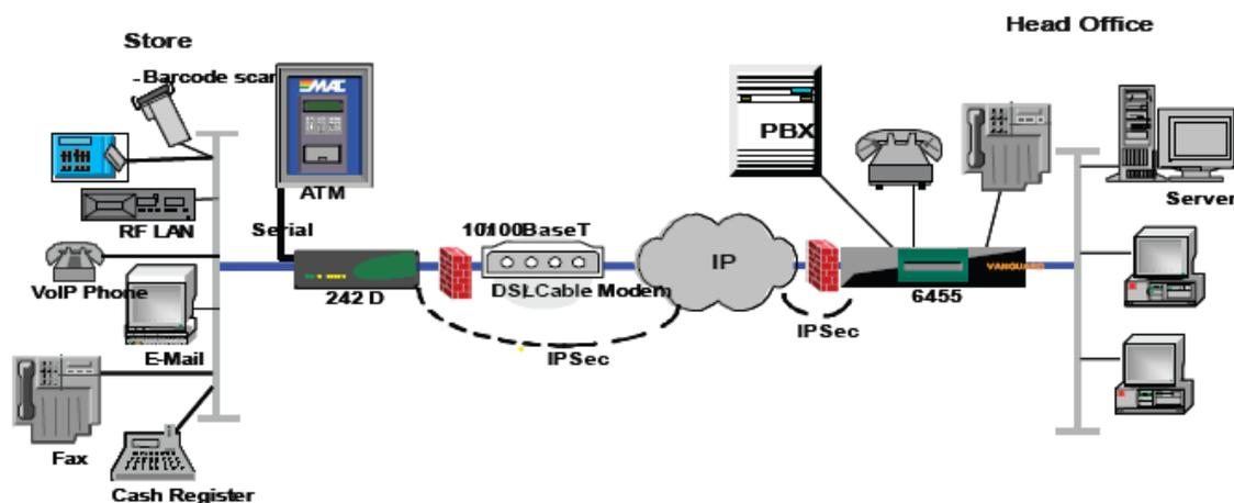
In this configuration, one LAN port is utilized to support in-store transactions while the second LAN port is used for secure Internet access through a DSL or cable modem connection. The serial port provides connectivity to a downstream ATM machine running a legacy serial protocol.
